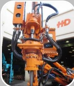
\* High Torque Double Head With 13,800 ft.lb Torque Bottom Head
