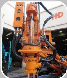
30' Sliding Stroke Between Two Heads
