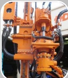
Heavy duty Hydraulic Side Shift Device for Double Head
