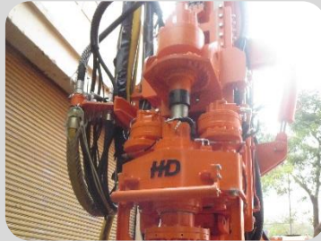
* High Torque Double Head With 45,000 ft.lb Torque Bottom Head
